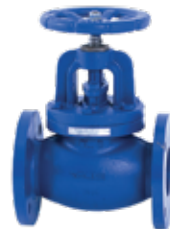
OS&Y GATE VALVE MSS SP-70 Cast Iron ASTM A-216 Gr.B FF Ends Class: 125 Sizes: 2" - 12" Fig. 144BR
